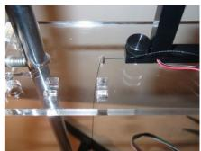
**Step 3:** Pass the thread through the eyebolt on the pulley platform directly below.
