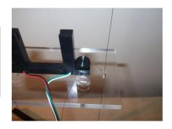
**Step 9:** Hook one of the pendulums onto the thread between the center eyebolts on the pendulum platform. Adjust the length of the string so that the center of the pendulum sits in the photogate sensor. Tighten the photogate screw.
