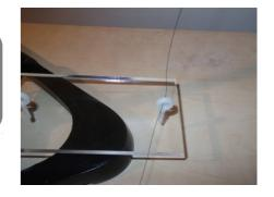
**Step 8:** Pass the thread back up through the same hole in the photogate platform and loosely wrap the thread around the thumb screw on the right-side of the photogate.
