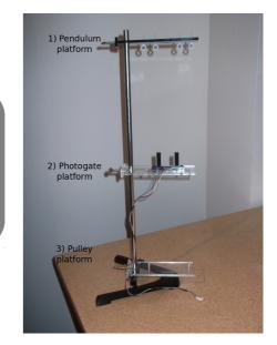
**Step 2:** Loosen the thumb screw on the leftside of the photogate. Wrap one end of pendulum thread around the thumb screw and tighten the screw down. Pass the other end of the thread through the adjacent hole in the photogate platform.
