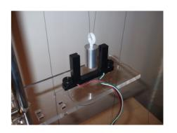
Step 10: Connect the photogate cable to the white 4-pin header on the sensor expansion board and plug the 9V battery clip into the board. Pull the pendulum back a small angle and release. As the pendulum swings through the photogate the period will be displayed.
