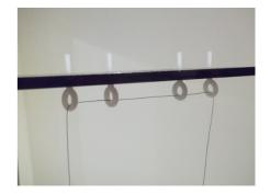
**Step 6:** Pass the thread down through the hole on the rightside of the photogate platform.
